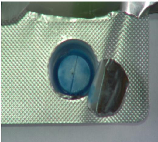
**Figure 5. Typical results of blue dye testing a pocket containing a 50µm laser drilled defect**
