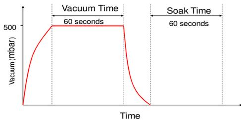
**Figure 3. Blue dye testing vacuum cycle**
