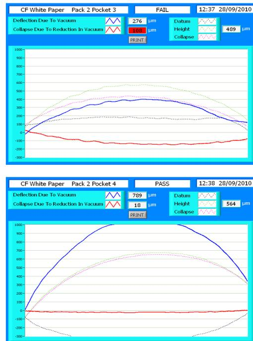
**Figure 2. BlisterScan results of a pack containing a 15µm hole (top) and a defect free pack (bottom).**
