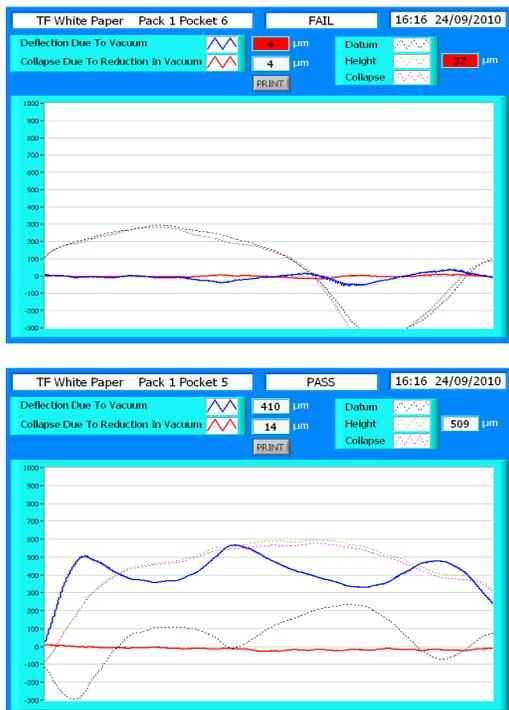
**Figure 1. BlisterScan results of a pack containing a 30µm hole (top) and a defect free pack (bottom).**
