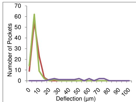
**Figure 7, BlisterScan data illustrating variation in collapse between defect free packs (green line) and those containing 12µm holes (red line) and 20µm holes (blue line)**
