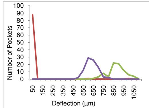
**Figure 6, BlisterScan data illustrating variation in deflection between defect free packs (blue line) and those containing 12µm holes (green line) and 20µm holes (red line)**
